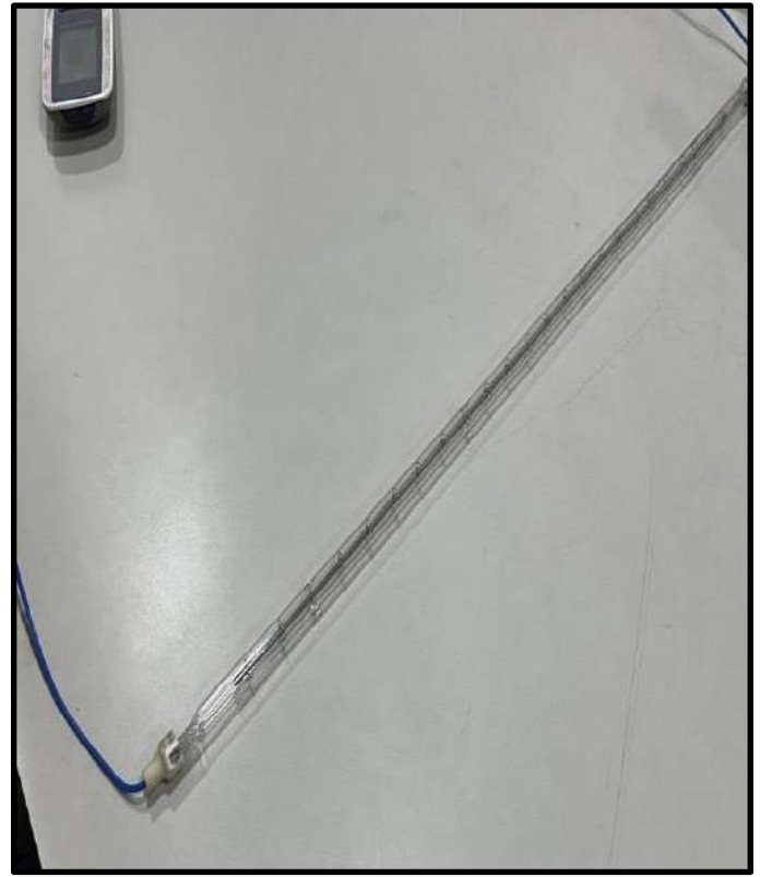
Picture 6.2: An infrared leaning rod manufactured by Litel
