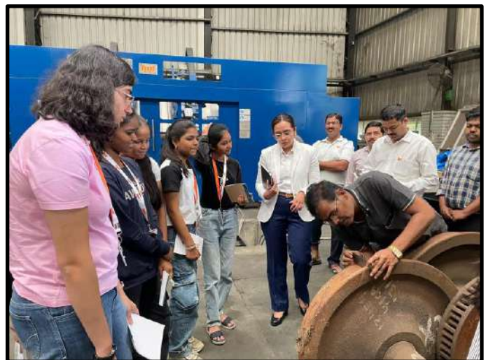
Picture 2.4: Ms Rajashri explains the process of measuring the railway wheel before it is cleaned in the CNC Portal Lathe
